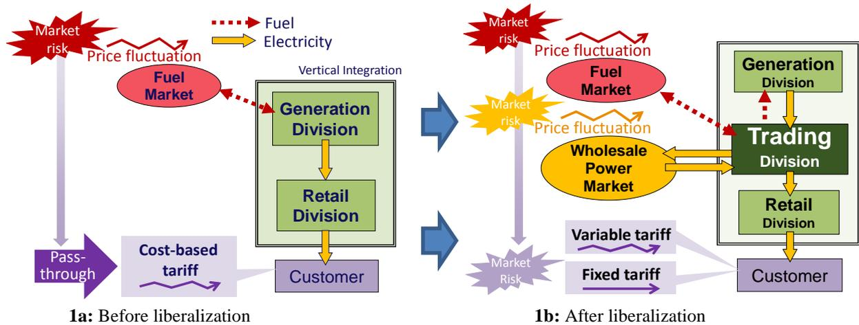
**Figure 1:** Change of the internal transaction of electricity in the power companies
