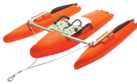
b) Tethered boat mounted with ADCP and STARFIRE WDGPS
