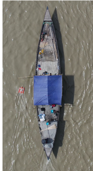
f) Aerial view of manned boat, tethered boat mounted with ADCP and WDGPS
